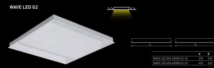
LED luminaires for offices and educational institutions. Thanks to the design and location of the optical part, as well as the use of lenses with a scattering angle 60 degrees, WAVE LED G2 luminaires have both high performance in efficiency up to 120 lm/W and unified glare rating UGR<16. Modifications with three or two light stripes, as well as different type of ceiling systems and edges, dimensions, power and color temperature are available on request.
